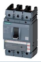
circuit breaker 3VA5 UL frame 250 breaking capacity class C 100kA @ 480V 3-pole, line protection TM210, FTFM, In=70A overload protection Ir=70A fixed short-circuit protection Ii=10 x In UL 489 SB (naval), 50 °C without connection
