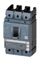
circuit breaker 3VA5 UL frame 250 breaking capacity class C 100kA @ 480V 3-pole, line protection TM210, FTFM, In=70A overload protection Ir=70A fixed short-circuit protection Ii=10 x In without connection
