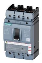
circuit breaker 3VA5 UL frame 250 breaking capacity class C 100kA @ 480 V 3-pole, line protection TM230, FTAM, In=70A overload protection Ir=70A fixed short-circuit protection Ii=5...10 x In cable connection load side
