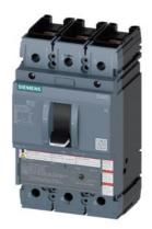
circuit breaker 3VA5 UL frame 250 breaking capacity class C 100kA @ 480 V 3-pole, line protection TM230, FTAM, In=70A overload protection Ir=70A fixed short-circuit protection Ii=5...10 x In UL489 SB load side
