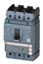
circuit breaker 3VA5 UL frame 250 breaking capacity class C 100kA @ 480 V 3-pole, line protection TM230, FTAM, In=70A overload protection Ir=70A fixed short-circuit protection Ii=5...10 x In nut keeper kit Al-lug, line and load side
