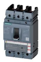
circuit breaker 3VA5 UL frame 250 breaking capacity class C 100kA @ 480V 3-pole, line protection TM230, FTAM, In=70A overload protection Ir=70A fixed short-circuit protection Ii=5...10 x In without connection
