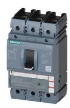
circuit breaker 3VA5 UL frame 250 breaking capacity class H 65kA @ 480 V 3-pole, line protection TM230, FTAM, In=70A overload protection Ir=70A fixed short-circuit protection Ii=5...10 x In nut keeper kit both sides
