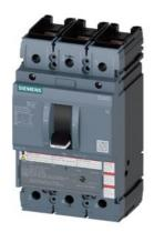
circuit breaker 3VA5 UL frame 250 breaking capacity class M 35kA @ 480 V 3-pole, line protection TM210, FTFM, In=70A overload protection Ir=70A fixed short-circuit protection Ii=10 x In UL489 SB (naval), 50 keeper kit on both sides
