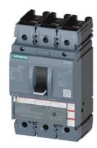
circuit breaker 3VA5 UL frame 250 breaking capacity class M 35kA @ 480 V 3-pole, line protection TM230, FTAM, In=70A overload protection Ir=70A fixed short-circuit protection Ii=5...10 x In nut keeper kit both sides
