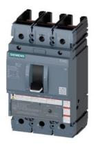
circuit breaker 3VA5 UL frame 250 breaking capacity class M 35kA @ 480V 3-pole, line protection TM230, FTAM, In=70A overload protection Ir=70A fixed short-circuit protection Ii=5...10 x In UL 489 SB (naval), 50 °C without connection
