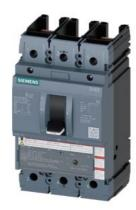
Circuit breaker 3VA5 UL Frame 250 Breaking capacity class C 100kA @ 480 V 2-pole, line protection TM210, FTFM, In=50A Overload protection Ir=50A fixed Short-circuit protection li=10 x In Without connection
