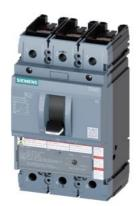
circuit breaker 3VA5 UL frame 250 breaking capacity class C 100kA @ 480 V 3-pole, line protection TM210, FTFM, In=50A overload protection Ir=50A fixed short-circuit protection Ii=10 x In UL489 SB (naval), 50 deg. cel. cable connection on both sides
