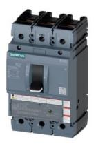
circuit breaker 3VA5 UL frame 250 breaking capacity class C 100kA @ 480 V 3-pole, line protection TM210, FTFM, In=50A overload protection Ir=50A fixed short-circuit protection Ii=10 x In UL489 SB (naval), 50 on both sides
