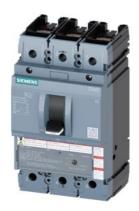
circuit breaker 3VA5 UL frame 250 breaking capacity class H 65kA @ 480 V 3-pole, line protection TM210, FTFM, In=50A overload protection Ir=50A fixed short-circuit protection Ii=10 x In UL489 SB (naval), 50 (naval), 50 deg. cel. cable connection on both sides
