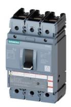
circuit breaker 3VA5 UL frame 250 breaking capacity class H 65kA @ 480 V 3-pole, line protection TM210, FTFM, In=50A overload protection Ir=50A fixed short-circuit protection li=10 x In cable connection on deg. cel. cable connection on both sides
