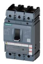
circuit breaker 3VA5 UL frame 250 breaking capacity class H 65kA @ 480 V 3-pole, line protection TM210, FTFM, In=50A overload protection Ir=50A fixed short-circuit protection Ii=10 x In nut keeper kit on on both sides
