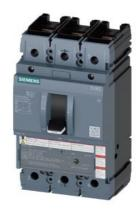
circuit breaker 3VA5 UL frame 250 breaking capacity class M 35kA @ 480 V 3-pole, line protection TM210, FTFM, In=50A overload protection Ir=50A fixed short-circuit protection Ii=10 x In UL489 SB (naval), 50 both sides
