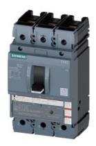
circuit breaker 3VA5 UL frame 250 breaking capacity class M 35kA @ 480 V 3-pole, line protection TM210, FTFM, In=45A overload protection Ir=45A fixed short-circuit protection Ii=10 x In UL489 SB (naval), 50 both sides
