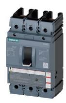
Circuit breaker 3VA5 UL Frame 250 Breaking capacity class C 100kA @ 480 V 2-pole, line protection TM210, FTFM, In=40A Overload protection Ir=40A fixed Short-circuit protection li=10 x In Without connection
