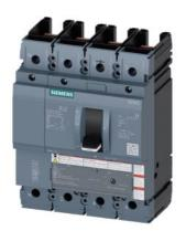
Circuit breaker 3VA5 UL Frame 250 Breaking capacity class C 100kA @ 480 V 4-pole, line protection TM210, FTFM, In=40A Overload protection Ir=40A fixed Short-circuit protection Ii=10 x In N conductor Unprotected Without connection
