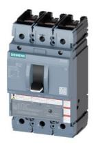
circuit breaker 3VA5 UL frame 250 breaking capacity class C 100kA @ 480 V 3-pole, line protection TM210, FTFM, In=40A overload protection Ir=40A fixed short-circuit protection Ii=10 x In UL489 SB (naval), 50 both sides
