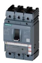
circuit breaker 3VA5 UL frame 250 breaking capacity class C 100kA @ 480 V 3-pole, line protection TM210, FTFM, In=40A overload protection Ir=40A fixed short-circuit protection Ii=10 x In nut keeper kit on on both sides
