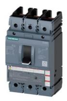
Circuit breaker 3VA5 UL Frame 250 Breaking capacity class C 100kA @ 480 V 3-pole, line protection TM210, FTFM, In=40A Overload protection Ir=40A fixed Short-circuit protection Ii=10 x In Without connection
