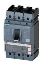
circuit breaker 3VA5 UL frame 250 breaking capacity class H 65kA @ 480 V 3-pole, line protection TM210, FTFM, In=40A overload protection Ir=40A fixed short-circuit protection Ii=10 x In nut keeper kit on deg. cel. nut keeper kit on both sides
