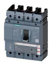
Circuit breaker 3VA5 UL Frame 250 Breaking capacity class M 35kA @ 480 V 4-pole, line protection TM210, FTFM, In=40A Overload protection Ir=40A fixed Short-circuit protection Ii=10 x In N conductor Unprotected Without connection
