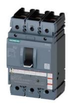
circuit breaker 3VA5 UL frame 250 breaking capacity class M 35kA @ 480 V 3-pole, line protection TM210, FTFM, In=40A overload protection Ir=40A fixed short-circuit protection Ii=10 x In UL489 SB (naval), 50 both sides
