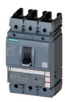
Circuit breaker 3VA5 UL Frame 250 Breaking capacity class M 35kA @ 480 V 3-pole, line protection TM210, FTFM, In=40A Overload protection Ir=40A fixed Short-circuit protection li=10 x In UL489 SB (naval), 50 deg. Cel Without connection
