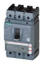
circuit breaker 3VA5 UL frame 250 breaking capacity class C 100kA @ 480 V 3-pole, line protection TM230, FTAM, In=250A overload protection Ir=250A fixed short-circuit protection li=5...10 x In nut keeper kit on both sides
