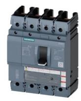
circuit breaker 3VA5 UL frame 250 breaking capacity class H 65kA @ 480V 4-pole, line protection TM240, ATAM, In=250A overload protection Ir=200A...250A short-circuit protection Ii=5...10 x In N conductor protection 100% without connection
