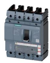
circuit breaker 3VA5 UL frame 250 breaking capacity class H 65kA @ 480V 4-pole, line protection TM230, FTAM, In=250A overload protection Ir=250A fixed short-circuit protection Ii=5...10 x In N conductor protection 100% without connection
