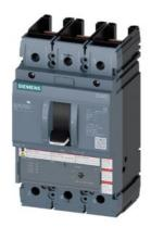
Circuit breaker 3VA5 UL Frame 250 3-pole, starter protection TM120M, AM, In=250A Without overload protection Short-circuit protection li=3...6 x In Without connection
