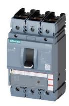
circuit breaker 3VA5 UL frame 250 3-pole, starter protection TM120M, AM, In=200A without overload protection short-circuit protection li=6...12 x In cable connection on both sides
