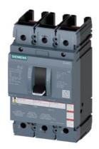
molded case switch 3VA5 UL frame 250 max. sh-circ breaking capacity 65kA @ 480V 2-pole, line protection MCS110, In=250A without overload protection self-protection li=10 x In without connection
