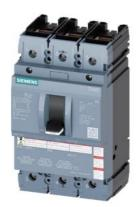
molded case switch 3VA5 UL frame 250 max. sh-circ breaking capacity 65kA @ 480 V 3-pole, line protection MCS110, In=250A without overload protection self-protection li=10 x In cable connection on both sides
