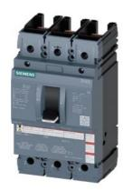
molded case switch 3VA5 UL frame 250 max short-circuit curr. rating 65kA @ 480 V 3-pole MCS110, In=250A without overload protection SELF PROTECTION Ii=10 x In Al-lug, line side
