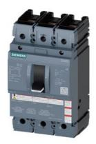
molded case switch 3VA5 UL frame 250 max. sh-circ breaking capacity 65kA @ 480 V 3-pole, line protection MCS110, In=250A without overload protection self-protection li=10 x In nut keeper kit on both sides
