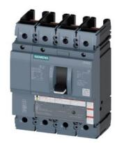
circuit breaker 3VA5 UL frame 250 breaking capacity class C 100kA @ 480V 4-pole, line protection TM210, FTFM, In=225A overload protection Ir=225A fixed short-circuit protection Ii=10 x In N conductor protection 100% without connection
