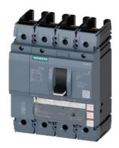
circuit breaker 3VA5 UL frame 250 breaking capacity class C 100kA @ 480V 4-pole, line protection TM230, FTAM, In=225A overload protection Ir=225A fixed short-circuit protection li=5...10 x ln N conductor protection 100% without connection
