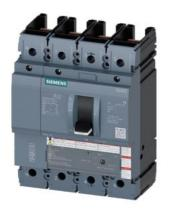
circuit breaker 3VA5 UL frame 250 breaking capacity class C 100kA @ 480V 4-pole, line protection TM230, FTAM, In=225A overload protection Ir=225A fixed short-circuit protection Ii=5...10 x In N conductor unprotected without connection
