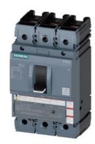
circuit breaker 3VA5 UL frame 250 breaking capacity class H 65kA @ 480 V 3-pole, line protection TM210, FTFM, In=225A overload protection Ir=225A fixed short-circuit protection Ii=10 x In UL489 SB (naval), 50 deg. cel. nut keeper kit on both sides
