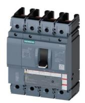
circuit breaker 3VA5 UL frame 250 breaking capacity class H 65kA @ 480V 4-pole, line protection TM230, FTAM, In=225A overload protection Ir=225A fixed short-circuit protection Ii=5...10 x In N conductor unprotected without connection
