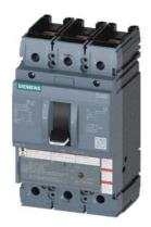
circuit breaker 3VA5 UL frame 250 breaking capacity class H 65kA @ 480 V 3-pole, line protection TM230, FTAM, In=225A overload protection Ir=225A fixed short-circuit protection Ii=5...10 x In nut keeper kit on both sides
