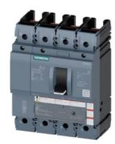
circuit breaker 3VA5 UL frame 250 breaking capacity class M 35kA @ 480V 4-pole, line protection TM210, FTFM, In=225A overload protection Ir=225A fixed short-circuit protection Ii=10 x In N conductor protection 100% without connection
