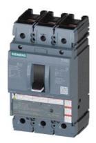
circuit breaker 3VA5 UL frame 250 breaking capacity class C 100kA @ 480 V 3-pole, line protection TM230, FTAM, In=200A overload protection Ir=200A fixed short-circuit protection li=5...10 x In nut keeper kit on both sides
