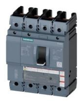
circuit breaker 3VA5 UL frame 250 breaking capacity class H 65kA @ 480V 4-pole, line protection TM240, ATAM, In=200A overload protection Ir=160A...200A short-circuit protection Ii=5...10 x In N conductor protection 100% without connection
