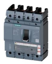
circuit breaker 3VA5 UL frame 250 breaking capacity class H 65kA @ 480V 4-pole, line protection TM230, FTAM, In=200A overload protection Ir=200A fixed short-circuit protection Ii=5...10 x In N conductor protection 100% without connection
