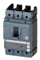
circuit breaker 3VA5 UL frame 250 breaking capacity class H 65kA @ 480V 2-pole, line protection TM210, FTFM, In=200A overload protection Ir=200A fixed short-circuit protection Ii=10 x In without connection
