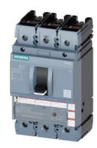
circuit breaker 3VA5 UL frame 250 breaking capacity class H 65kA @ 480 V 3-pole, line protection TM210, FTFM, In=200A overload protection Ir=200A fixed short-circuit protection Ii=10 x In UL489 SB (naval), 50 deg. cel. cable connection on both sides
