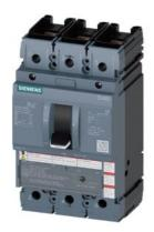
circuit breaker 3VA5 UL frame 250 breaking capacity class H 65kA @ 480 V 3-pole, line protection TM210, FTFM, In=200A overload protection Ir=200A fixed short-circuit protection Ii=10 x In nut keeper kit on both sides
