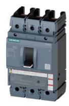
circuit breaker 3VA5 UL frame 250 breaking capacity class H 65kA @ 480V 3-pole, line protection TM210, FTFM, In=200A overload protection Ir=200A fixed short-circuit protection Ii=10 x In UL 489 SB (naval), 50° C without connection
